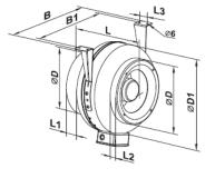
**Note:** Typical fan for 300i is a pre-wired, three-pronged plug VKM 200. Two fans needed. Call factory for special pressure drops or applications.
